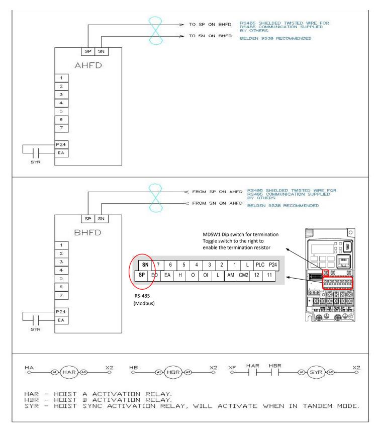
EZCOM wiring example circuit. Make sure the BVFD has the RS485 termination resistor dip switch toggled to the right.
