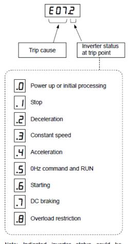
Note: Indicated inverter status could be different from actual inverter behavior. e.g. When PID operation or frequency given by analog signal, although it seems constant speed, acceleration and deceleration could be repeated in very short cycle.
